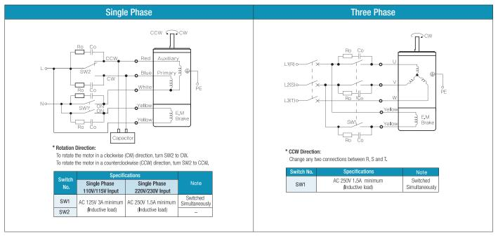
1) The direction of motor rotation is as viewed from the shaft end of the motor.
