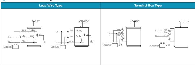
1) The direction of motor rotation is as viewed from the shaft end of the motor.
