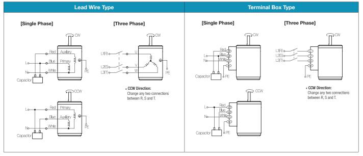
1) The direction of motor rotation is as viewed from the shaft end of the motor.
