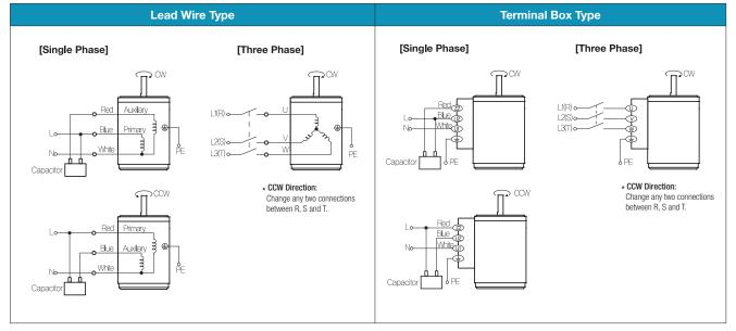
1) The direction of motor rotation is as viewed from the shaft end of the motor.
